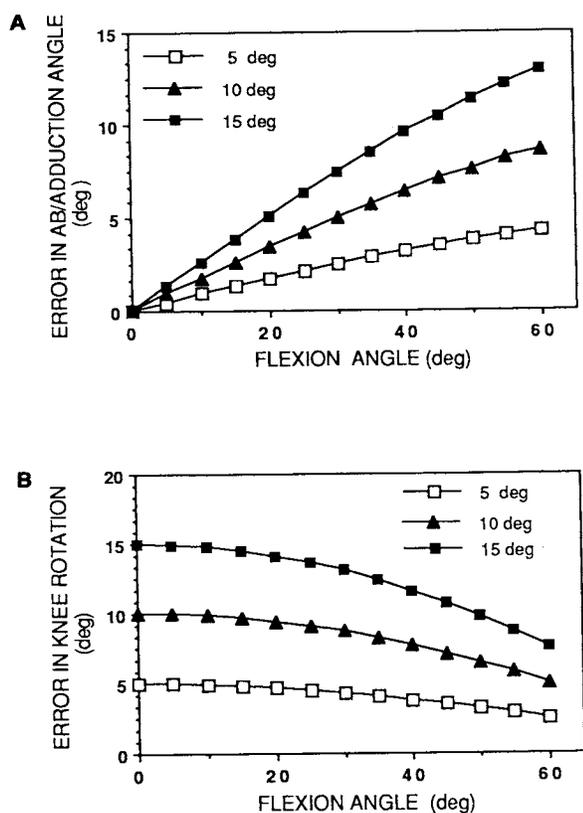
FIG. 7. Error in knee varus/valgus angle (A) and rotation angle (B) as a function of knee flexion angles for errors in the definition of knee flexion-extension axis.
