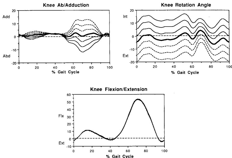
**FIG. 6.** Errors in the definition of embedded axes on knee angles. All angles are in degrees. Thick line indicates the measured joint angles of a representative subject. The flexion-extension axis is analytically rotated through a range of -15 to +15° from the reference position in steps of 5°. Corresponding knee angles are plotted in thin lines.
