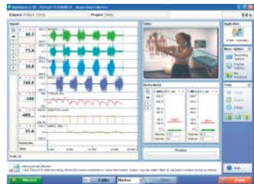
Fig. 4: Direct look into the body / muscle function: EMG synchronized with video and other movement sensors. Software screenshot of MyoResearch XP™ - NORAXON INC. USA
