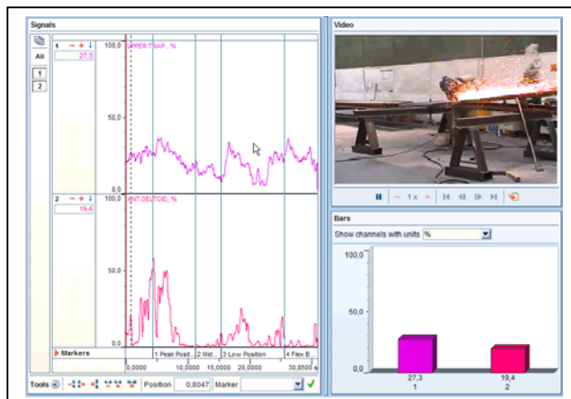
Fig. 76: Ergonomic EMG analysis of two shoulder muscles (upper trace -: trapezius p. desc; lower trace - deltoideus anterior) in a work task within a steel production process. The MVC normalized signal show the muscular demand in ratio to the given video picture
