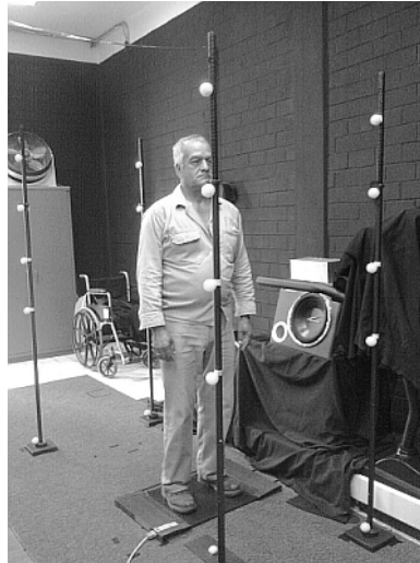
Figure 18: The subject was submitted to an infrasonic stimulation laterally at the hip
