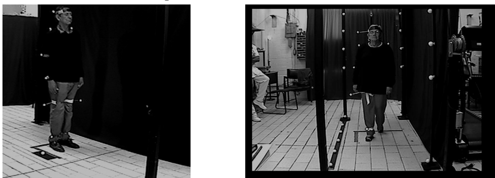
Figure 9: A 71 years old man and an 83 years old woman under study, reflective markers fixed to the main joints and head in the calibrated volume are shown.
